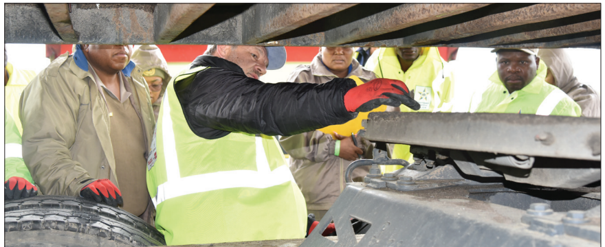
▲ Manie Roux of Jost is passionate about 5th Wheels and explains to officers their function and what can go wrong. And things do go wrong. A small crack can lead to a cascade of events.
