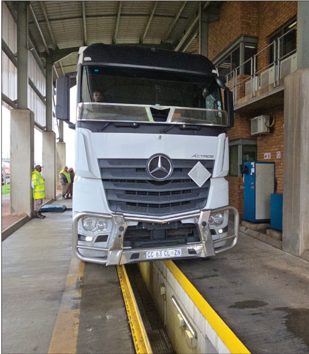
▲ One of the two rigs that were randomly selected for inspection seen here over the pit in the test centre. It is here that the teams of traffic officers are led through various stages of inspection with accent on easily identifying faults that could deem a rig to be unroadworthy. This one passed.
